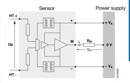
In the same way as for current sensors, this secondary current  $I_{\mbox{\tiny S}}$  can be then passed through a measuring resistance  $R_{\mbox{\tiny M}}.$  The measuring voltage  $V_{\mbox{\tiny M}}$  at the terminals of this measuring resistance  $R_{\mbox{\tiny M}}$  is therefore also exactly proportional to the primary voltage  $U_{\mbox{\tiny P}}.$  The electrical supply to the sensor is also insulated from the primary voltage.
