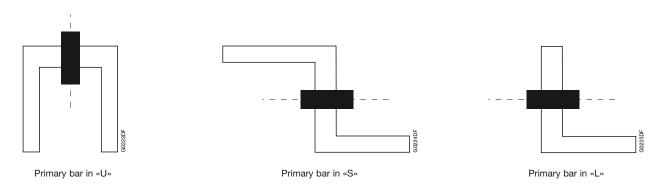
The tests were carried out with the primary bars in «U» configuration, the most restricting condition.
