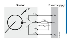
The secondary output voltage  $V_{\rm S}$  is therefore directly proportional to the primary current. It is an exact replica of the primary current, generally with a value of 4V for a nominal current  $I_{\rm PN}$ .
