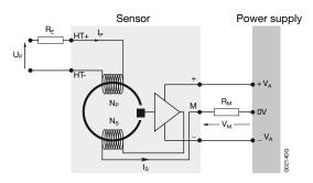
Principle diagram of a not calibrated EM010 sensor
