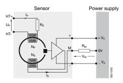
Principle diagram of a calibrated EM010 sensor
