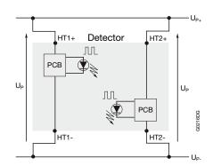
The voltage detector indicates the presence of a voltage higher than a limit (maximum 50V in compliance with standards) by the illumination of a LED. Inversely, the LED is extinguished when the voltage is below this limit.
