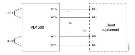
The two connections HT+ (client equipment side) must be made at different connection points. The two connections HT - (client equipment side) must be made at different connection points.
