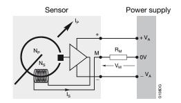
The secondary output current  $I_{\rm S}$  is therefore exactly proportional to the primary current at any moment. It is an exact replica of the primary current multiplied by the number of turns  $N_{\rm P}/N_{\rm S}$ . This secondary current  $I_{\rm S}$  can be passed through a measuring resistance  $R_{\rm M}$ . The measuring voltage  $V_{\rm M}$  at the terminals of this measuring resistance  $R_{\rm M}$  is therefore also exactly proportional to the primary current  $I_{\rm P}$ .
