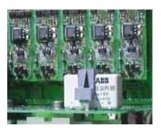
These sensors are designed for PCB mounting.
