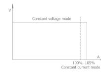
Rectangular current limit characteristic of Polyamp DC/DC converters
