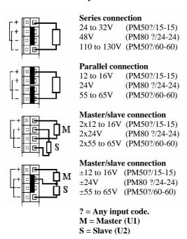
Figure 1. Output connections
