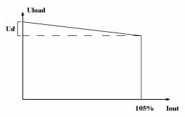
Figure 3. Load regulation with voltage drop  $U_{\rm d}$  between output and load
