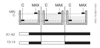
The CM-ENN monitors levels of conductive liquids and is used for example for liquid level monitoring in pump control systems, for dry-running protection of submersible pumps or overflow monitoring of tanks. It is also suitable for conductivity monitoring of liquids. The measuring principle is based on the resistance change sensed by single-pole electrodes (wet or dry).
