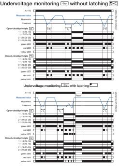
If the measured value exceeds resp. drops below the adjusted threshold value, the tripping delay T<sub>v</sub> starts. If T<sub>v</sub> is complete and the measured value is still exceeding resp. below the threshold value plus resp. minus the set hysteresis, the output relays energize 🖃 / de-energize 🖭.
