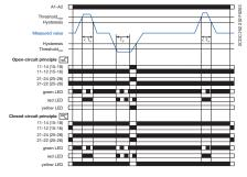
Voltage window monitoring 1x2 c/o contact 🔤 OFF-delayed **III** without latching 🔀
