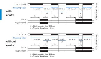
If all phases (and the neutral) are present, the output relay energizes after the start-up delay t\_ is complete. If a phase failure occurs, the tripping delay t\_ starts. When timing is complete, the output relay denergizes. As soon as the voltage returns to the tolerance range, timing of t\_ starts. When timing is complete, the output relay re-energizes automatically. The yellow LED glows when the output relay is energized.
